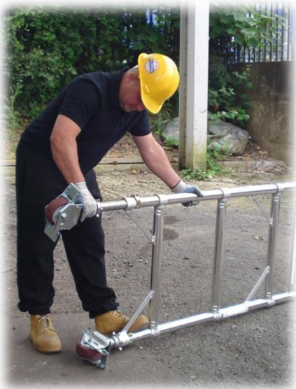
1. Insert 2 legs and castors into each frame.
